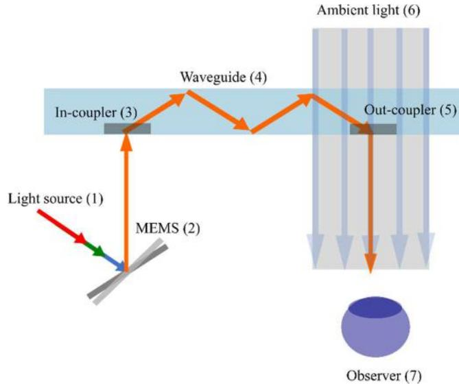
Figure 1: Schematic view of a LBS (1 and 2) coupled into a waveguide (4) in order to redirect the image to the observer (7).
