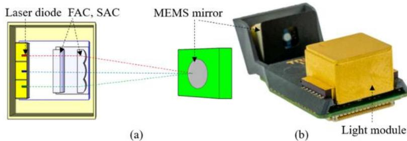
Figure 2: (a) Schematic and (b) image of a TriLite LBS – the Trixel<sup>®</sup><sup>17</sup>.
