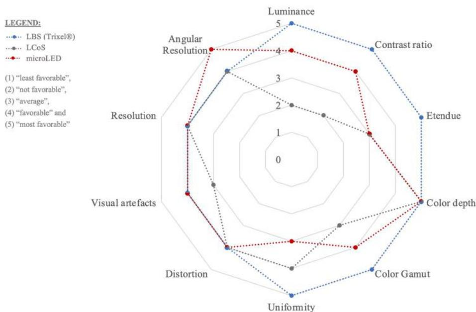
Figure 4: Image quality – benchmarking LBS, LCoS and mLED displays for XR glasses.
