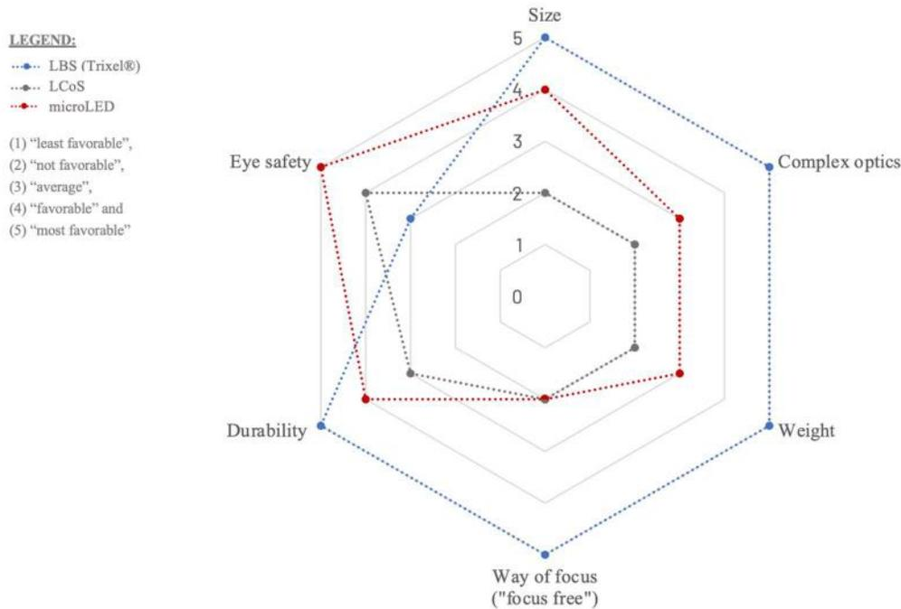
Figure 6: User aspects – benchmarking LBS, LCoS and mLED displays for XR glasses.
