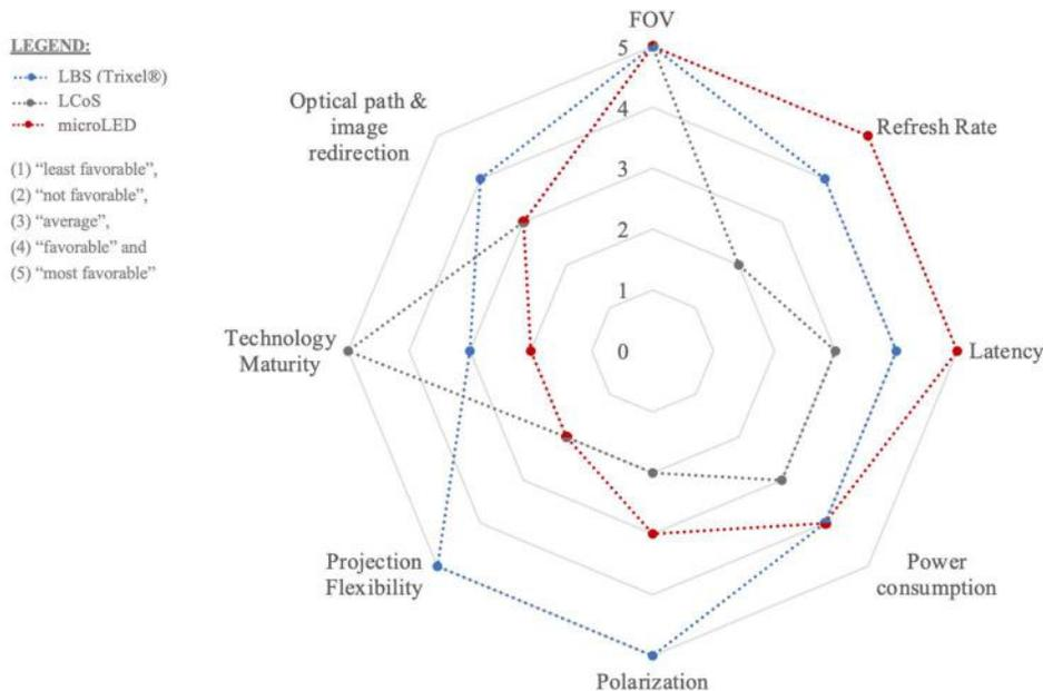
Figure 5: XR Display Characteristics– benchmarking LBS, LCoS and mLED displays for XR glasses.
