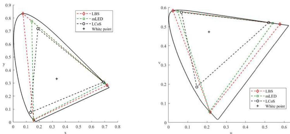
Figure 3: CIE 1931 and CIE 1976 gamut comparison between state-of-the-art LBS, LCoS and mLED.
